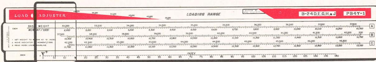
LOAD ADJUSTER SHOWING BASIC WEIGHT AND MOMENT SCALE
